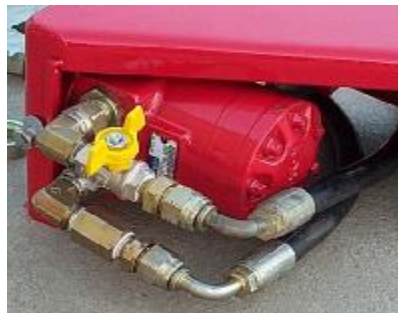
Figure 5 - Hoses fitted to motor
