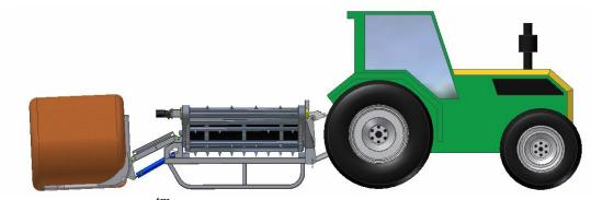
Lower the Bigeasy<sup>tm</sup> so that the skids are in contact with the ground or very close to it, this will ensure that the lift forks are the correct height when lowered to slide under the bale for safe effective loading. The forks should be driven under the bale until the bale makes contact with the upright of the lift forks.
